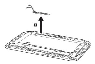
When installing: Route the antenna cables along the cable guides and secure the antenna boards with adhesive tapes. As you route the cables, make sure that they are not subjected to any tension. Tension could cause the cables to be damaged by the cable guides, or a wire to be broken.
